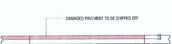
SECTION OF EXISTING PAVEMENT
